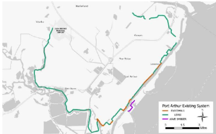
Figure 1. Location map of the Sabine to Galveston (S2G) Coastal Storm Risk Management (CSR) proposed project action areas including floodwalls (orange), levees (green), and wave barriers (purple).
