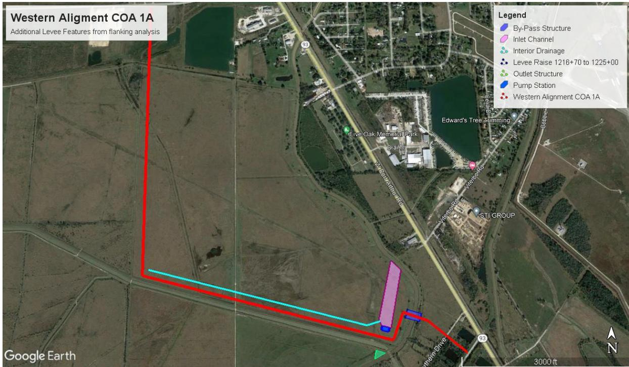
Figure 9-Western Levee Alignment COA 1-A and features
